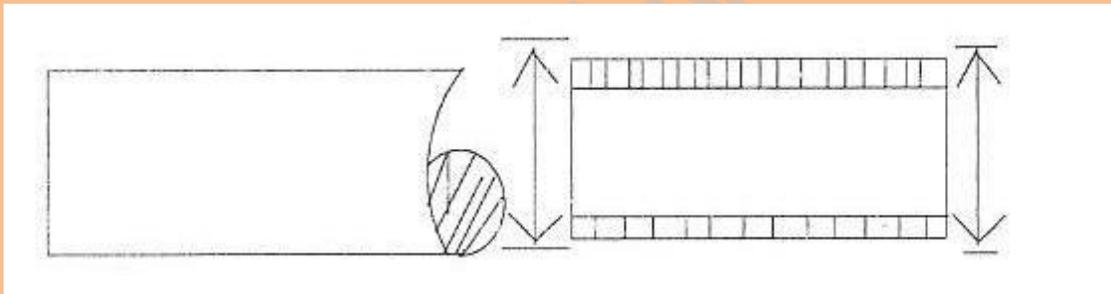
3. **Interference Fit:** This is the type of fit which exist between the shaft and a hole in such a way that the dimension on the shaft is more than that on the hole, force is required to couple the two parts together.
