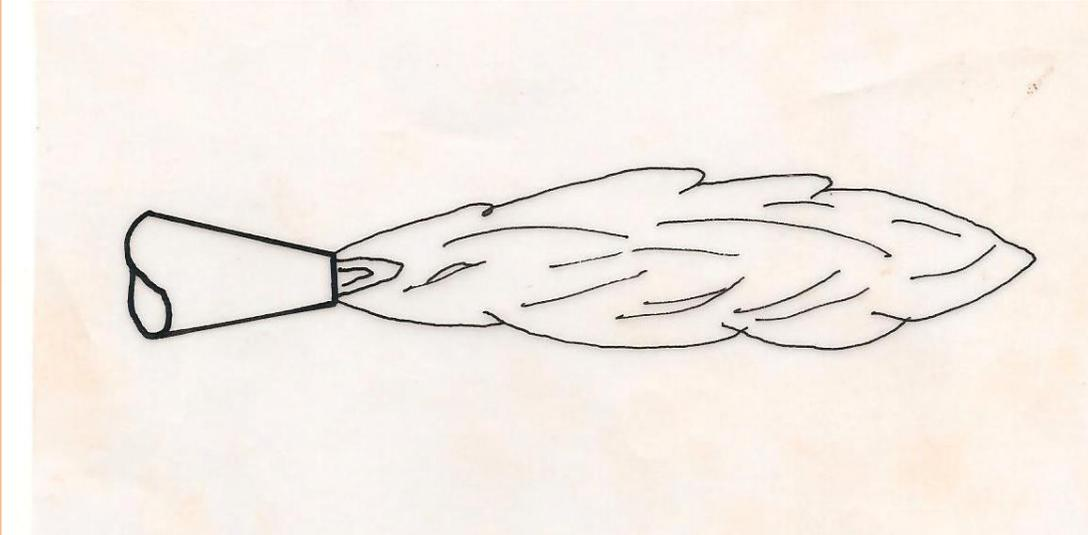
Application: It contains excess acetylene which results in carbon rich zone extending around and beyond the inner cone. It is used mainly for hard surfacing.
